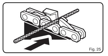
Using light but firm pressure, stroke towards the front corner of the tooth. Lift file away from the steel on each return stroke.
